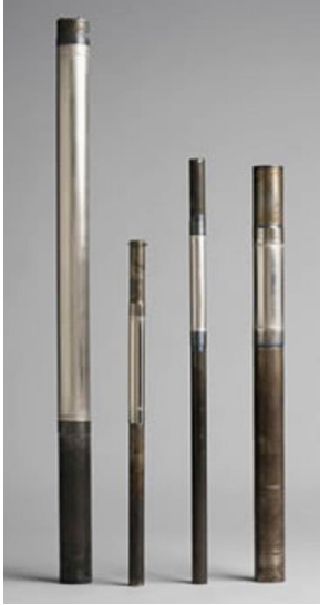
Figure 8: High-temperature Pd-based composite hydrogen separation membranes manufactured by CRI/criticatalyst.
