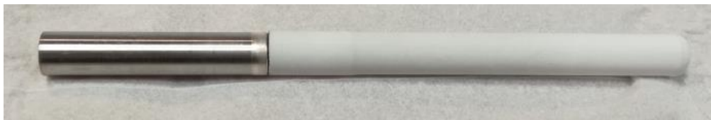
Figure 7. Porous ceramic tube welded to a metallic dense tube.
