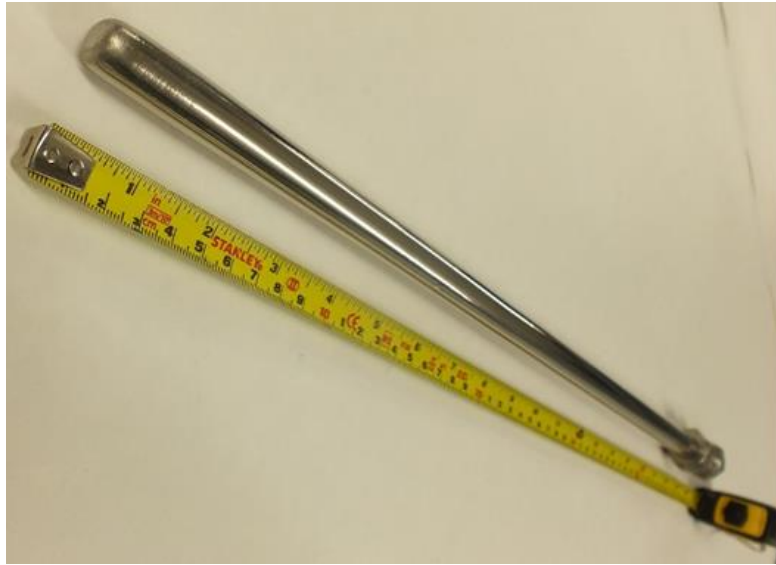
Figure 5. Finger type Pd-Ag membrane supported on porous alumina support.
