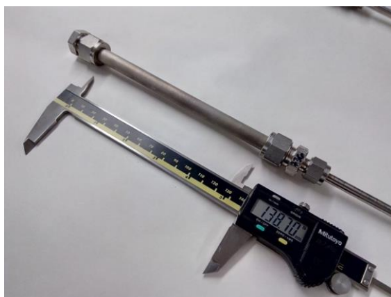
Figure 7. Pd-Ag membrane with an effective thickness layer between 2-3 \mu\text{m} , outer diameter of 10 mm and inner diameter of 7 mm.
