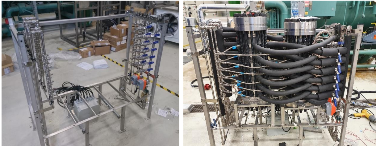
Figure 2. EHP stack frame for easy placement of stacks in the skid of the EHP sub-system.
