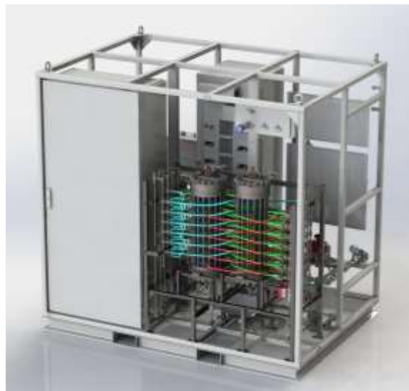
Figure 9. Render of the sub skid for the EHP stacks
