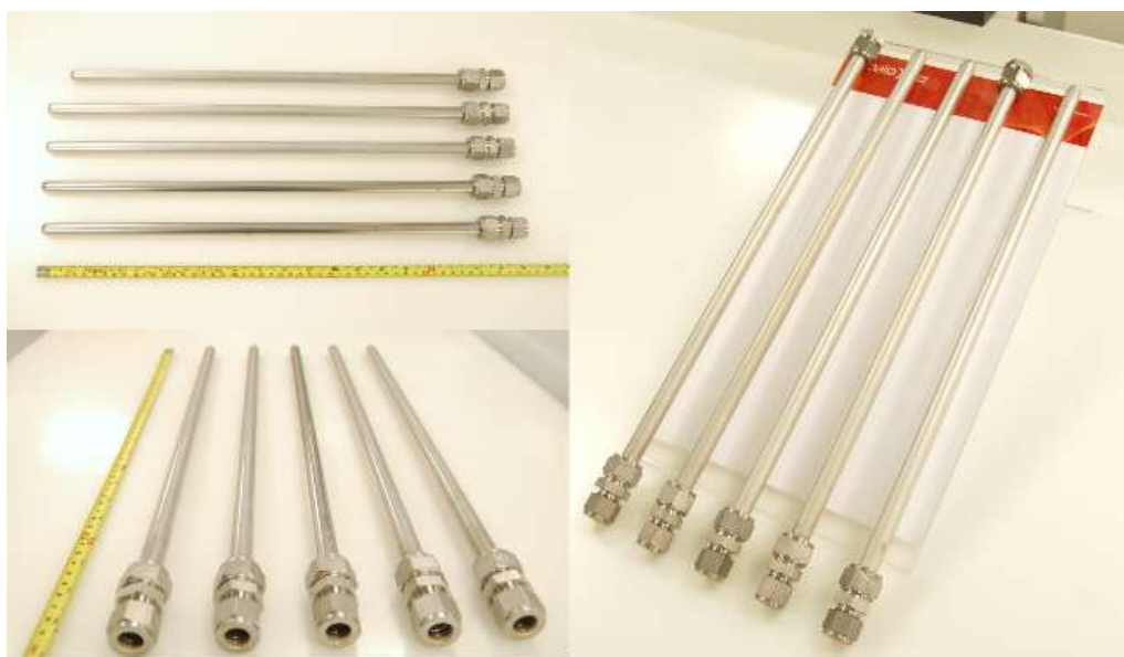
Figure 3. Pd-Ag ceramic supported membranes of 450 mm length.
