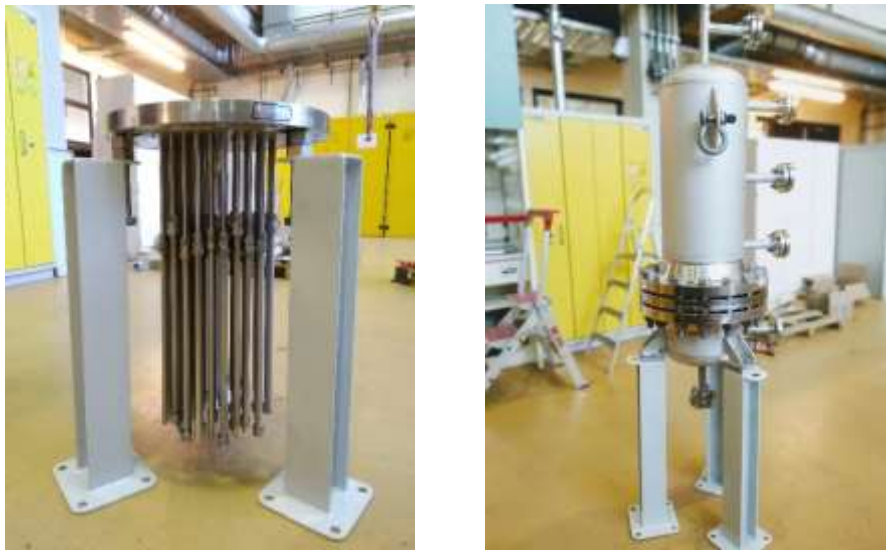
Figure 8. (left) The 66 Pd-Ag ceramic supported membranes already welded to the flange and ready to be integrated in the prototype and (right) HyGrid membrane module prototype after the membrane integration where all the flanges have been closed and the reactor is already face up.
