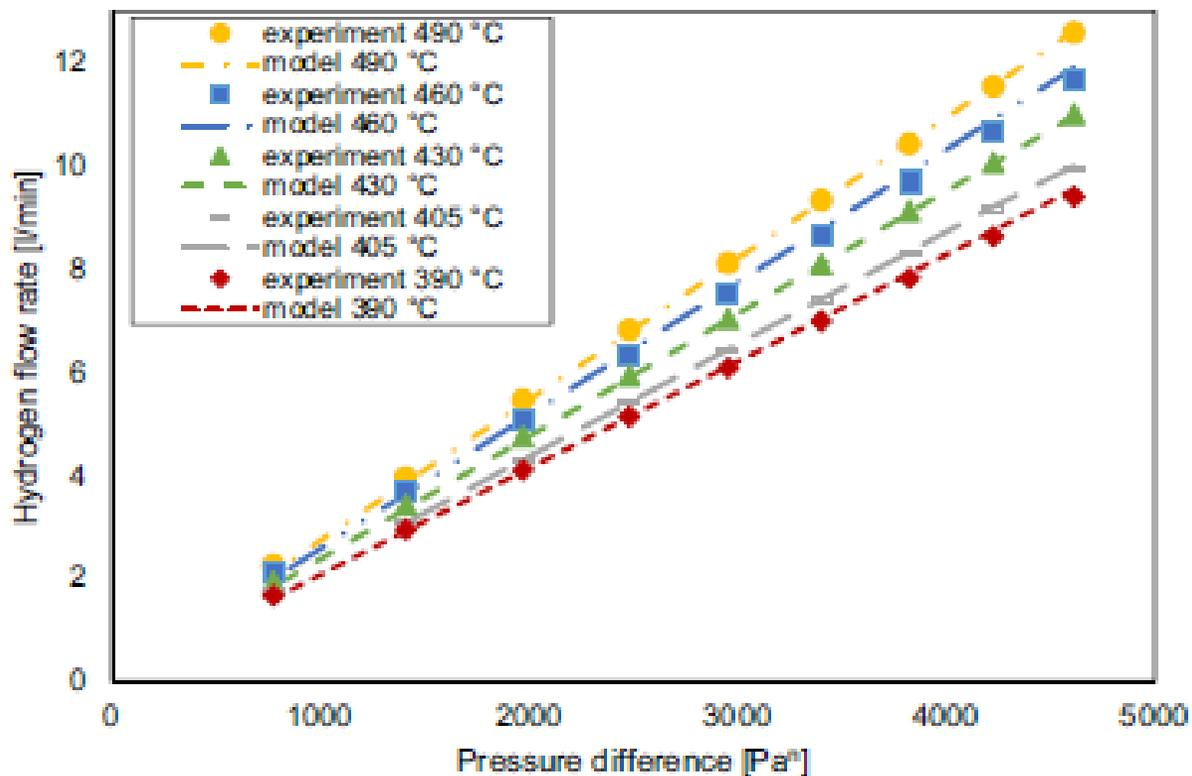
Experimental and modelled results in pure gas tests at different operating temperature with Pd2DS membrane.
