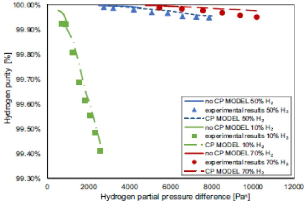
Hydrogen purity from experimental and modelled results in mixture tests at different hydrogen inlet content; continuous line to described ideal case and dotted line includes mas
