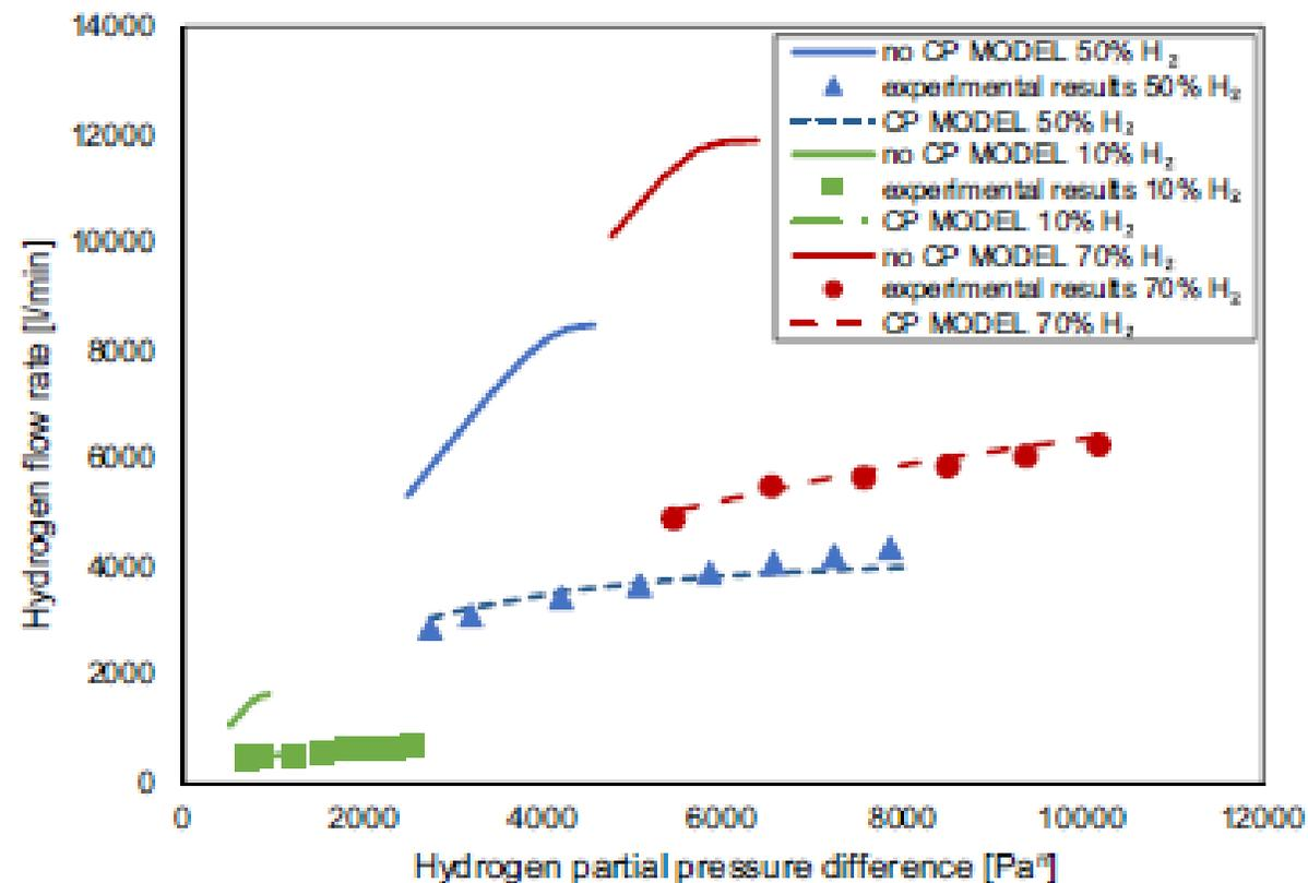
Hydrogen flux from experimental and modelled results in mixture tests at different hydrogen inlet content; continuous line to described ideal case and dotted line includes mass transfer limitation at a working temperature of 400 °C.
