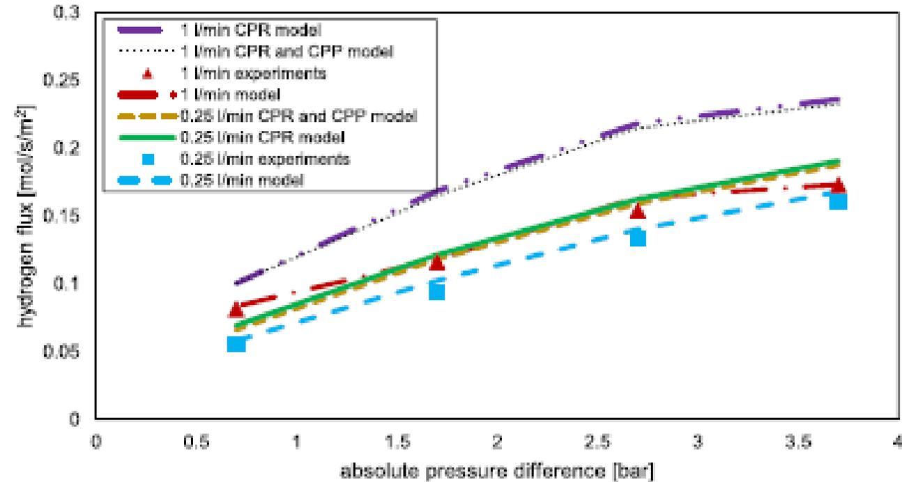
Comparison between experimental and modeling results for a mixture of  $\text{CH}_4/\text{H}_2$  with nitrogen as sweep gas. The sweep gas is 0.25 l/min.
